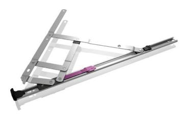
Initial opening similar to Standard Side Hung Friction Stay. Full opening to 90° providing clear egress in excess of 500 mm on a 600 mm wide vent. Easy to operate thumb catches allow the vent to slide to the easy clean position giving between 100 and 250 mm clear opening.
